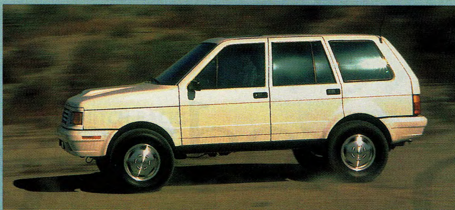
The 5250-pound truck is an intimidator on the road. However, it is also a formidable off-road warrior. The Laforza's frame, body and interior were designed and built in Turin, Italy and shipped to the U.S. where the Ford powertrain (engine and transmission) was installed by Cars & Concepts of Brighton, Michigan.
