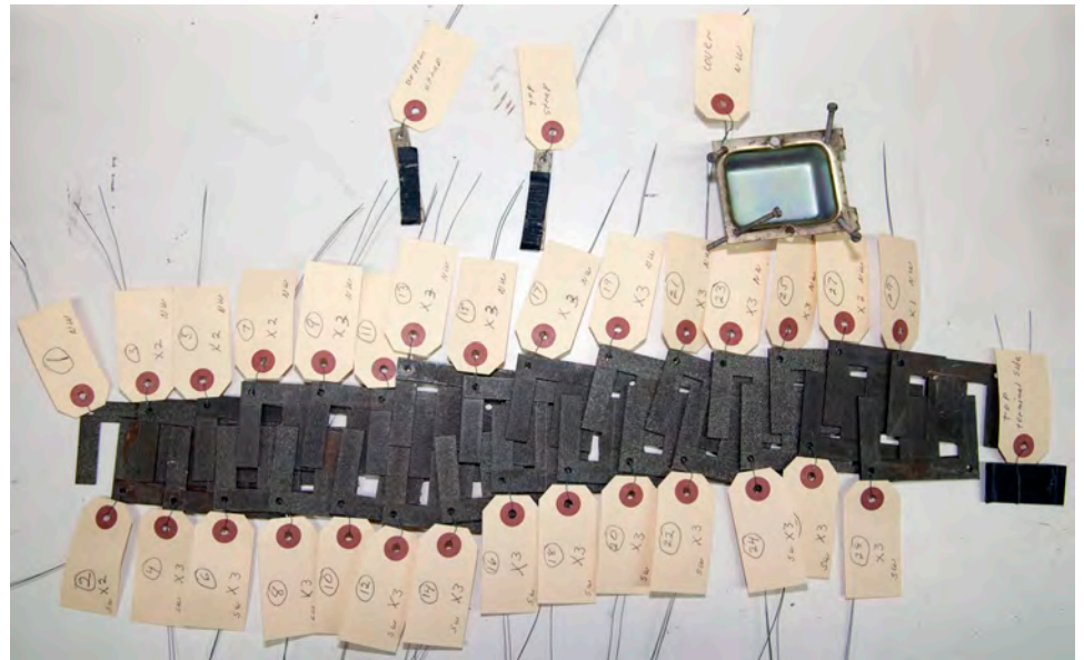
The AC15's transformer after it was fully disassembled.
