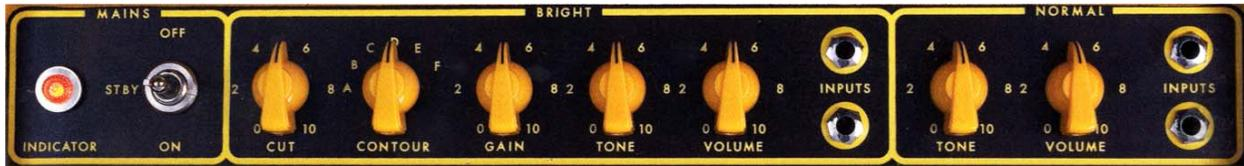
between two Gain controls mounted on the footswitch. Dual 1/4" input jacks (high and low gain) are provided for each channel, and a footswitch jack, as well as internal and external 1/4" speaker jacks with an impedance selector.
