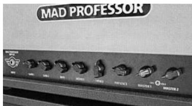
Controls are straight up – gain for channels one and two, bass, middle, treble, presence controls, a master volume for each
