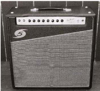
We received a 1x15 version of the 40 watt *Andrew*, which is also available in 2x10, 2x12 and 4x10 configurations. The 1x15 is equipped with our favorite current production 15" – the *Eminence Legend* – along with dual 5881 power tubes and an
