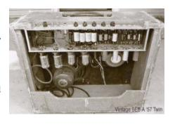
panel" cabinet with speakers mounted in each corner. In the next circuit revision (1956–57 model 5E8A), a ground switch was added and the treble tone circuit was removed from the negative feedback loop. Leo Fender couldn't play a lick on the guitar, but he obviously never stopped thinking about how to improve the sound and performance of his
