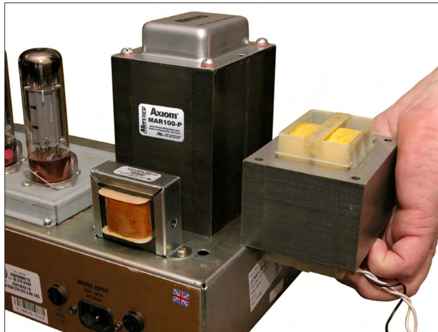
Mercury's Axiom MAR100-P transformer compared to the original Marshall iron.
